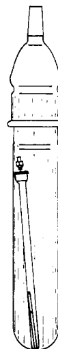
Figure 6. Arrangement for replacing the air inside the NMR tube by argon (see Experimental Section).
